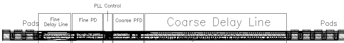
Figure 6.29 ADPLL chip layout
